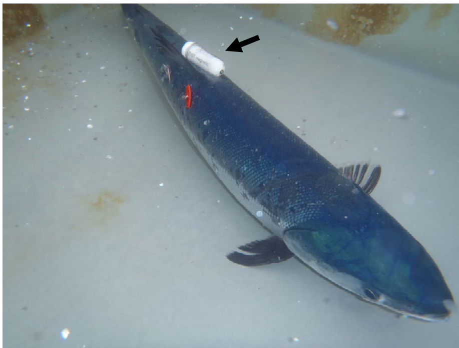
Fig. 2. Chum salmon tagged with an archival tag (arrow, DST magnetic manufactured by Star-Oddi) that measures and records earth's magnetic field strength (in three directions), tilt (in three directions), acceleration, temperature and depth.
