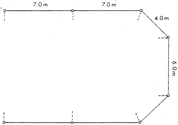
Fig.3 Arrangement of hanging ropes attached to the ground rope. The hanging ropes are 1.0 m each in length and were installed to lift the fishing rope up from the sea bottom at tow.
