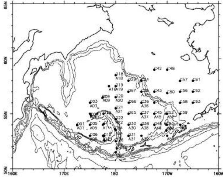
Figure 1. Observation points of R/V *Kaiyo maru* from June to September cruise in 2002. A represents observation points during leg 1, C represents observation points during leg 3, and D represents observation points during leg 4.
