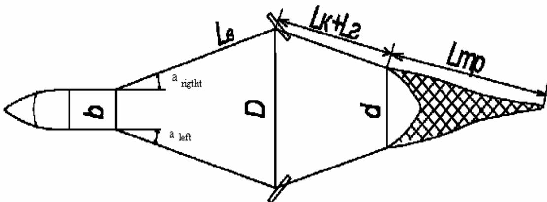
Fig. 4. Method for measuring divergence angle of warps
