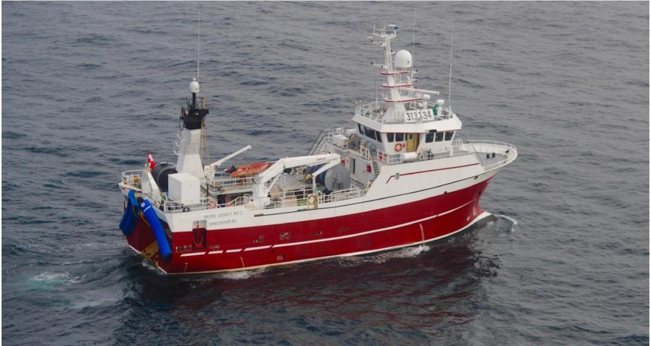
Photo: Canadian freezer trawler, Pacific Legacy. Pacific Legacy is 37m long, 10m beam, a draft of 6m, a gross tonnage of 600 t and 2600 horsepower.
